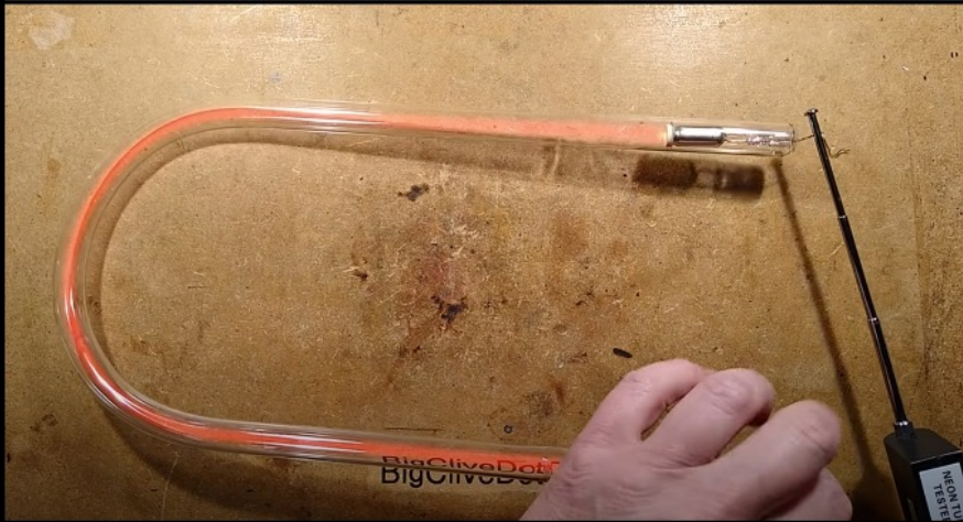
Using a high-voltage neon tube tester (spark coil) to illuminate tube units Screenshot: Youtube.com
