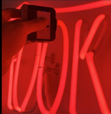
Photo-documentation of color is unreliable. Use a spectrometer to measure chromaticity
