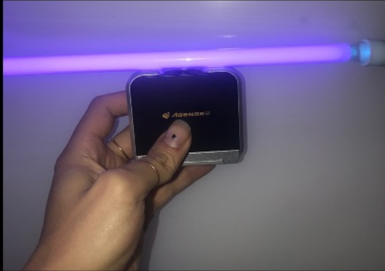
Capturing spectral measurements of a gas-discharge tube with an "Asensetek Lighting Passport" portable spectrometer
