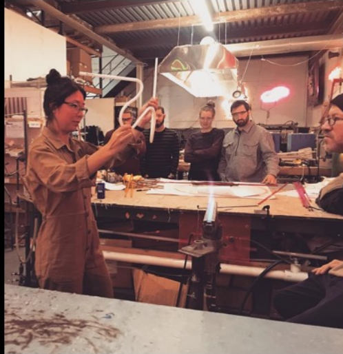
Using a ribbon burner to bend a glass tube during a fabrication workshop at Brooklyn Glass
