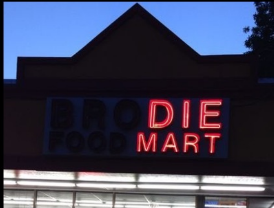
Electronic components fail as gas-discharge components age Brodie Food Mart in Austin, Texas becomes "Die Mart" Photo: FourSquare
